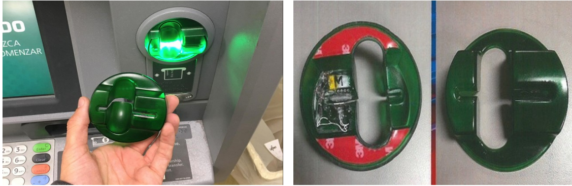
Figure 3: Showing a magnetic stripe skimming device found attached on an ATM machine [33]. The internal circuitry of the skimming device is also shown.
